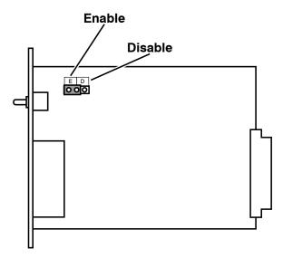
Figure 4.3: Circuit Module Jumper
